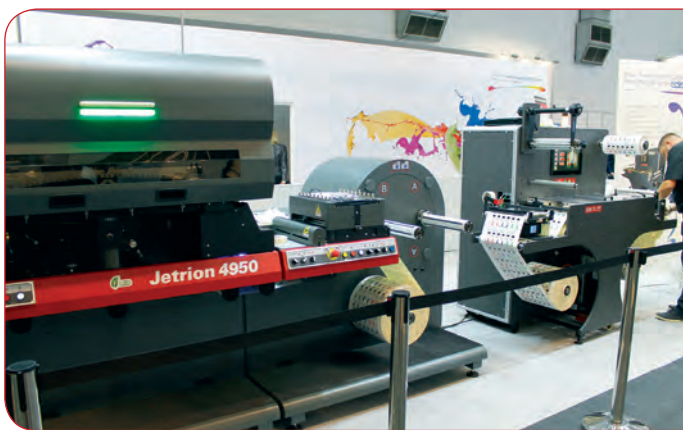
The TCC 3300 die-cutter is a new option for the EFI Jetrion press
