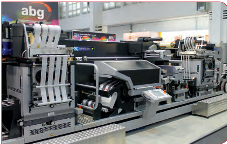
Digicon 3 line on the ABG stand with new flatbed screen-printing unit and two Bigfoot modules
